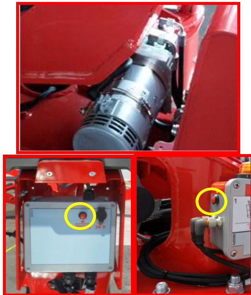
Picture 41: electropump (*optional) activation buttons.
