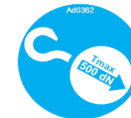
Picture 72: indication of frame coupling.
