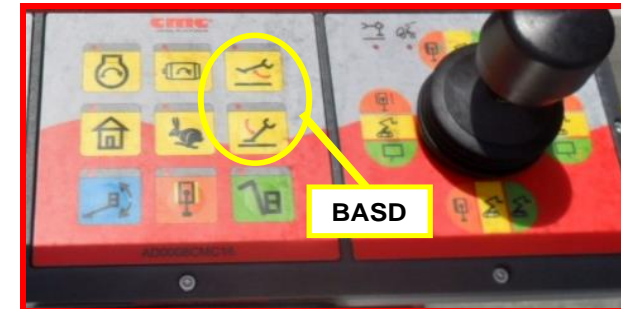
Picture 27: stabilization/destabilization buttons on basket station control.
