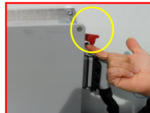
Picture 30: emergency bypass lever.
