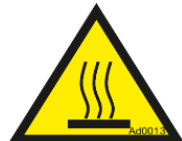
Picture 83: warning of burn risk.
