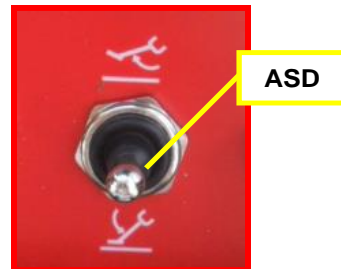
Picture 26: stabilization/destabilization lever on wired remote control.
