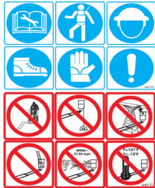
Picture 81: general obligations and prohibitions.
