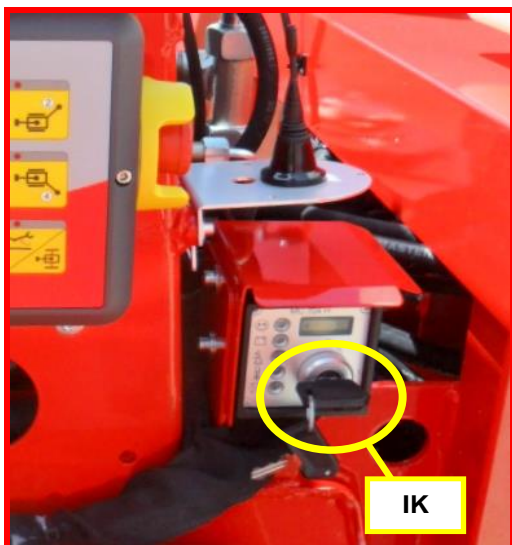
Picture 4: engine switch on/off station if Kubota.
