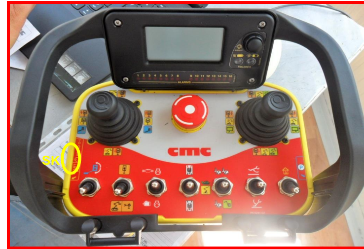
Picture 13: platform wired remote/radio control station.
