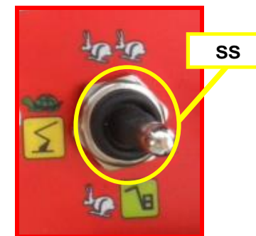
Picture 22: speed selector on wired remote control.
