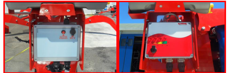
Picture 9b: basket electric box.
