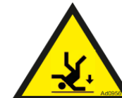
Picture 88: danger of falling.
