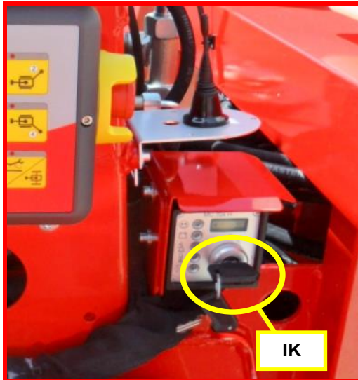
Picture 4: engine switch on/off station if Kubota.
