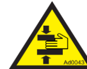
Picture 86: crushing and cutting hazard.
