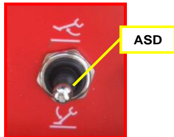
Picture 26: stabilization/destabilization lever on wired remote control.
