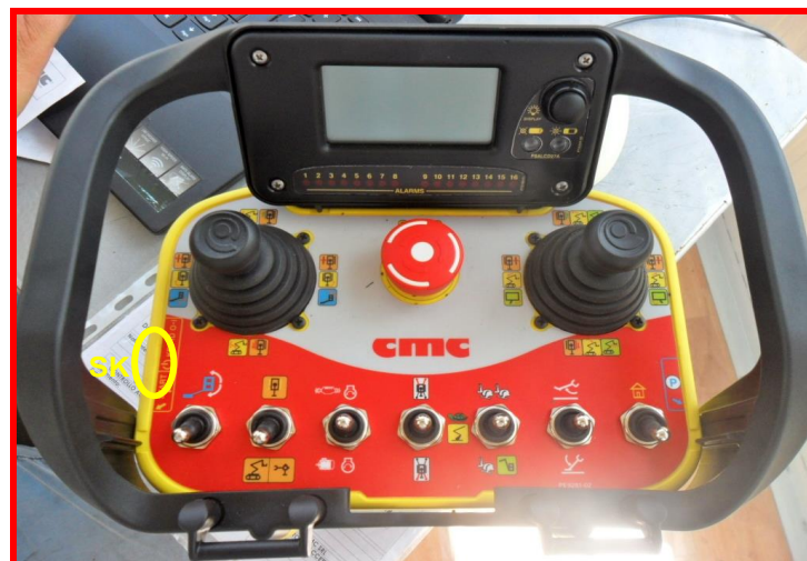
Picture 13: platform wired remote/radio control station.
