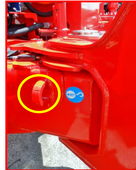
Picture 20: couplings on the frame.
