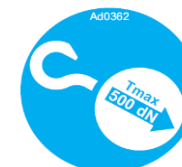
Picture 72: indication of frame coupling.
