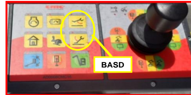
Picture 27: stabilization/destabilization buttons on basket station control.
